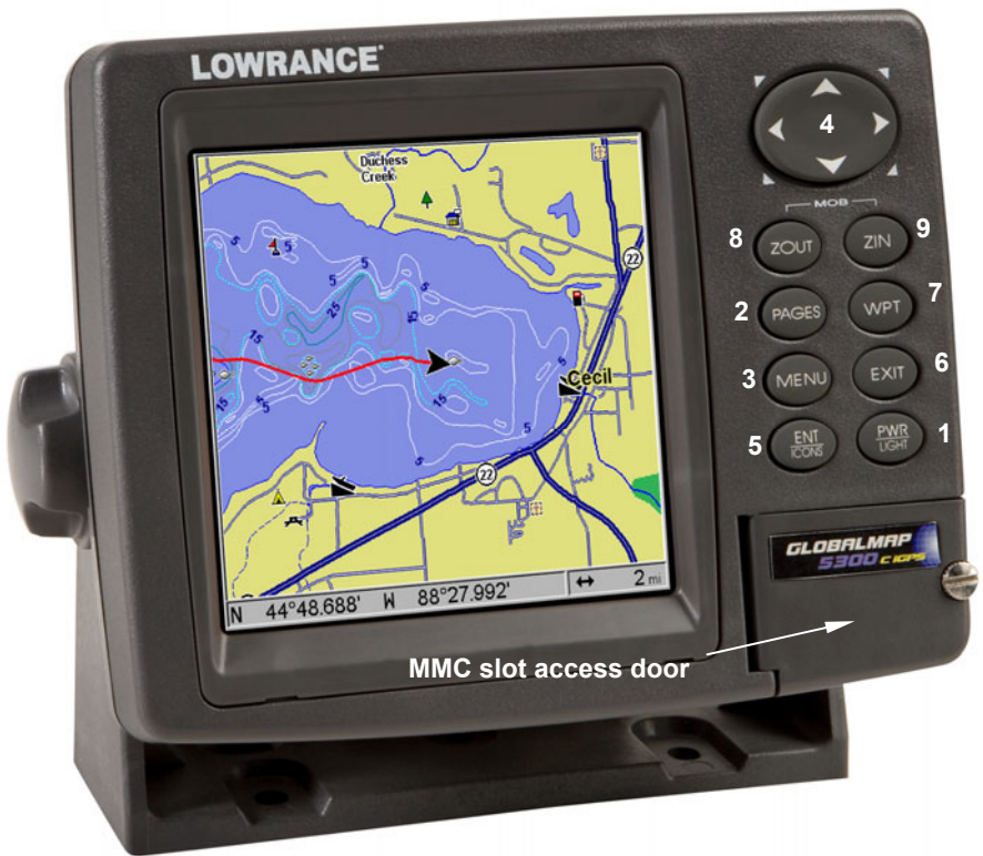
GlobalMap 5300c GPS unit, front view, showing Map Page, keyboard and access door for the MMC slot.
